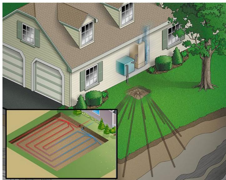
*Ground source heat pumps use the earth as a heat source in the winter or as a heat sink in the summer, benefiting from the earth's stable temperature.*
